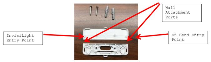
2. Attach the Indoor/Outdoor cable to the wall with Staples entering the right hand port and route a loop of fiber around the fiber management posts. Adhere the InvisiLight fiber to the wall with adhesive and enter the left hand port and route a loop of fiber around the fiber management posts leaving enough fiber to splice to the EZ Bend Indoor/Outdoor cable .
